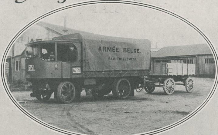
The "Sentinel" Steam Waggon can carry 6 tons safely at a speed of 10 miles an hour.
